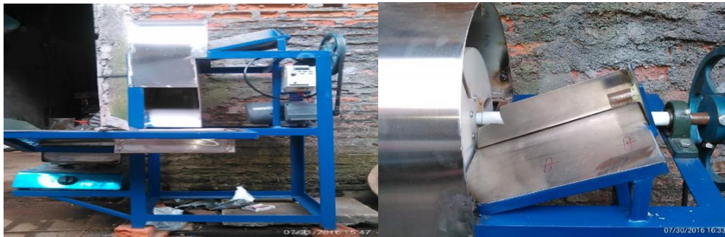
Figure 3. Multifunctional tempe slicing machine
