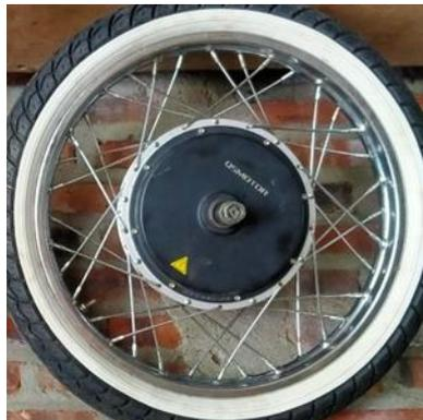
Gambar 1. Motor BLDC Type E-BIKE
