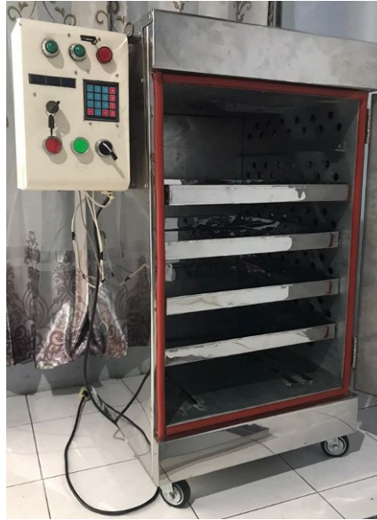
Figure 2. Multipurpose dryer with five trays and control panel for temperature and time settings.
