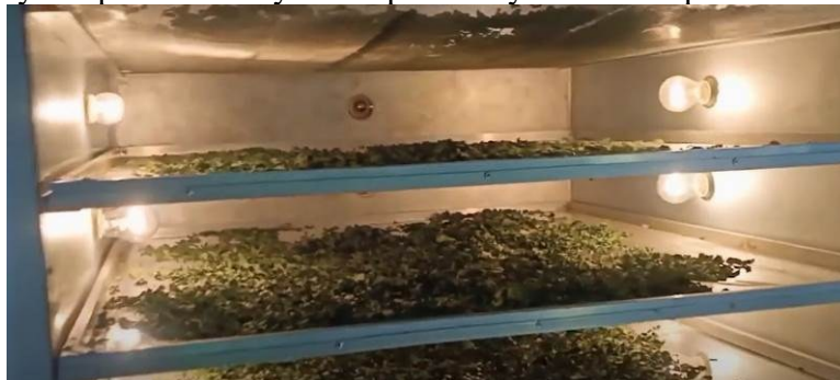
Figure 4. Drying results of moringa leaves showing even drying with consistent moisture levels.
