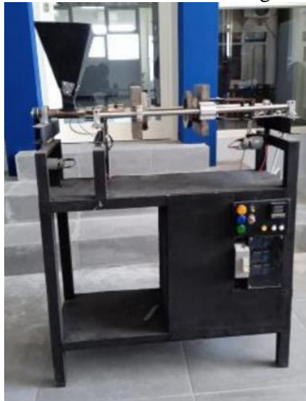
Figure 2. Plastic injection molding machine design.
