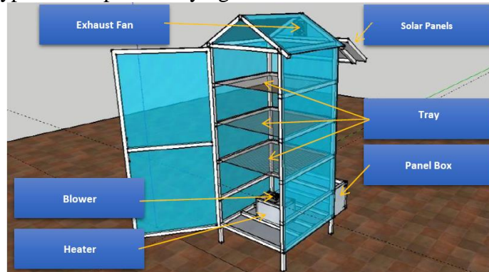
Figure 1. A Water Spinach ( Ipomoea Aquatica ) Vegetable Drying Chamber With A Spiral Type Heater.
